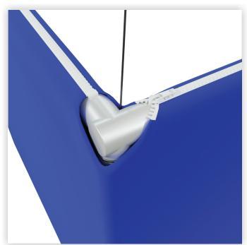
**Step 3**Pull the cable through the opening in the fabric.
